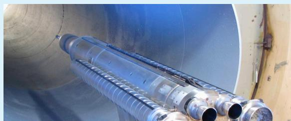
The SLS team has completed extensive wind tunnel testing at NASA's Ames Research Center in Moffett Field California, Langley, and Marshall. These tests use scale rocket models to study how the vibration, base heating, and other environments affect the launch vehicle designs for both the Block 1 and Block 1B SLS configurations.
